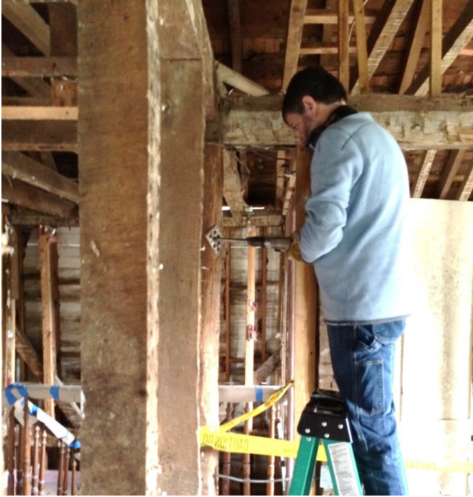
Michael Worthington of Oxford Tree-Ring Laboratory extracting samples to determine dates of construction.
